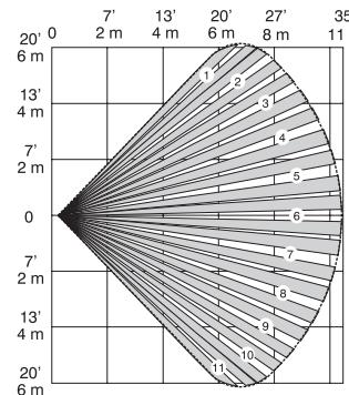
**Note :** The distances in the illustrations do not represent the maximum detection distances. A walk-test is required after mounting to ensure proper detection.
